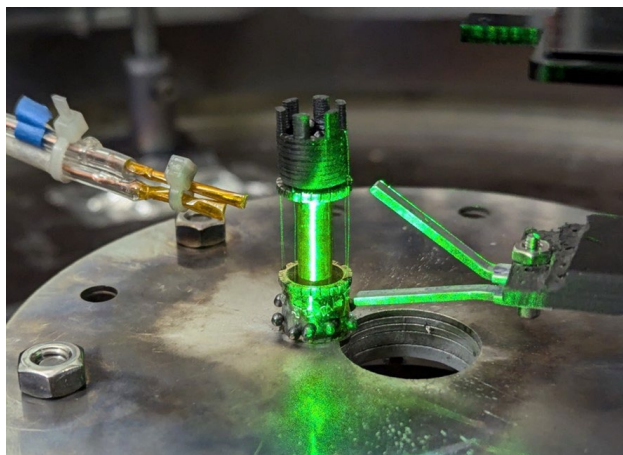
Figure 2. A photo of the load hardware showing the wire array (middle), b-dot probes (left), and the obstacle (right).
