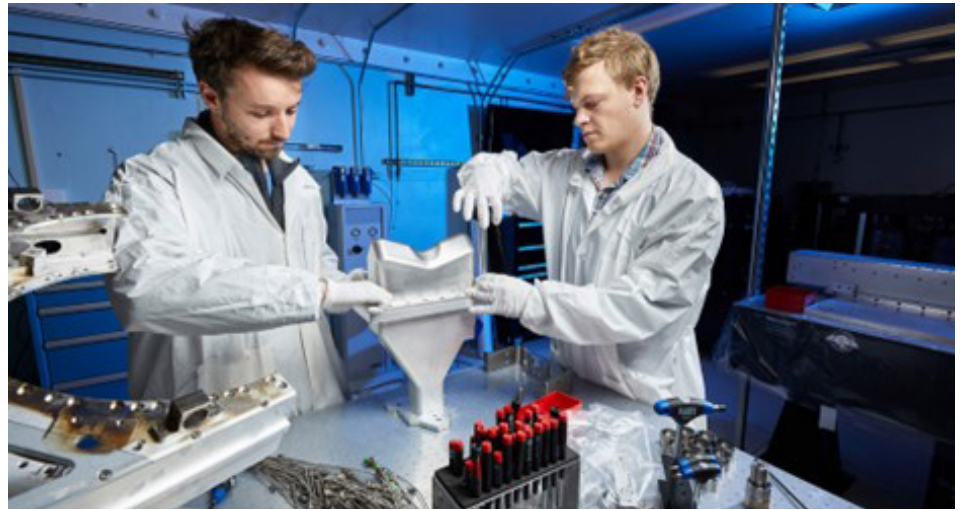
Figure 1. Lawrence Livermore researchers Eric Stern (left) and Kelton Grange work on the fielding hardware commissioned for use in NIF weapons survivability experiments. The steel case protects against the destructive force from significant amounts of X-rays and debris generated by megajoule-class inertial confinement fusion experiments. Credit: Garry McLeod/LLNL.
