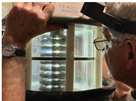
Long-time lab employee Harry Wilhelm, lead technician, checks the alignment of o-rings as he reassembles one of COBRA's self-break main switches.
