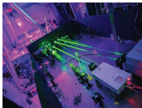
The image shows CESZAR, a 1 megaampere Linear Transformer Driver in the background with laser beam paths for a multi-channel interferometry system in the foreground.
