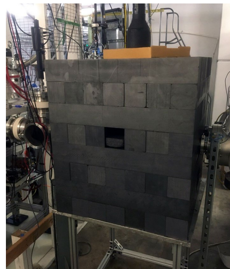
Figure 1. An 80-centimeter cube of graphite was used to moderate the neutrons produced by the Cyclotron Institute's K150 cyclotron. (Credit: Cyclotron Institute, Texas A&M University)
