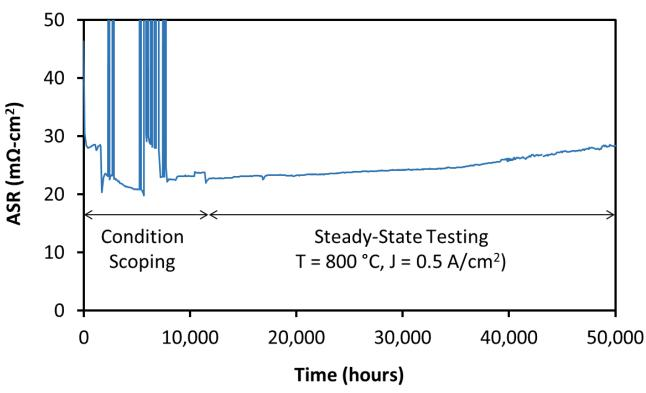
Nexceris' commercialized manganese cobalt oxide (MCO) coating technology to protect metallic interconnects from corrosion, which is critical for long stack life in SOFC and HTE applications.
