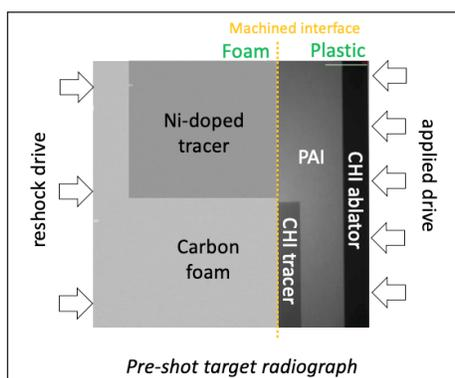
Figure 1: Pre-shot radiograph with the different materials and regions labeled. The direction of the applied drive and reshock drive are also labeled.
