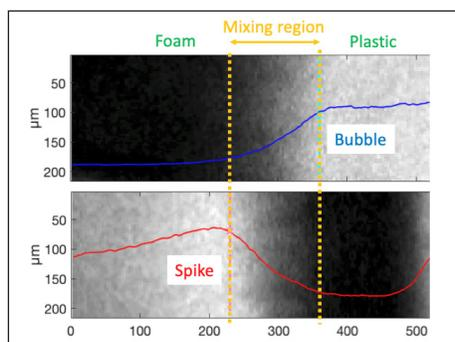
Figure 2: Experimental radiograph. The dashed lines mark bubble and spike front positions determined by where the contrast starts to transition from light to dark. The distance between the dashed lines is the width of the mixing region.
