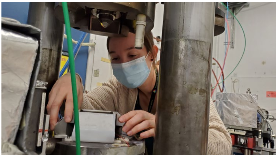
University of Nevada Las Vegas PhD student Taryn Traylor positioning the DDIA anvils in preparation for an experiment measuring the change in sound velocity of \text{SiO}_2 at high pressure under compressive stress. She is working at the Advanced Photon Source sector 6 (6BM-B) using the COMPRES supported multianvil apparatus.
