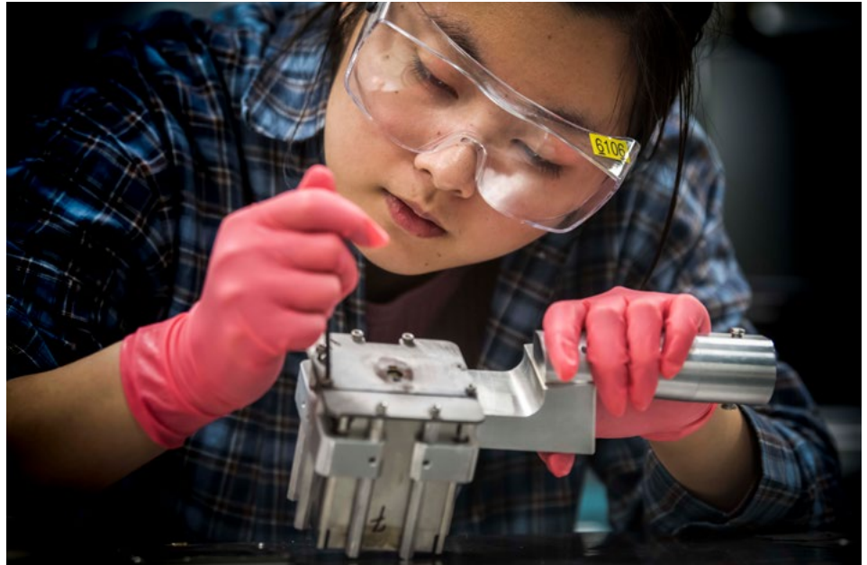
Figure 1. Zixuan Ye building a PXRDIIP box for a MgO shock compression experiment for her PhD thesis at Omega EP, Laboratory for Laser Energetics at Rochester University.
