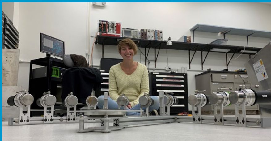
Rebecca Toomey with 10 deuterated liquid scintillator ODeSA neutron detectors. These detectors were mounted at the University of Notre Dame to measure the ^{18}\text{O}(\alpha, n) reaction that is important for nuclear non-proliferation and applications in geophysics and astrophysics. (p. 26)
