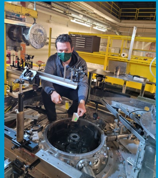
Kyle Swanson configuring vertical laser interferometry diagnostics for electron density measurements of photoionized supersonic gas jets on the Zebra pulsed-power accelerator. (p. 25)
