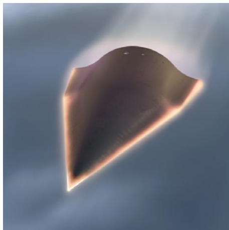
Figure 1. Illustration of a hypersonic glide vehicle, the Hypersonic Technology Vehicle 2, developed as part of the Defense Advanced Research Projects Agency (DARPA) Falcon project. (Image credit: DARPA).
