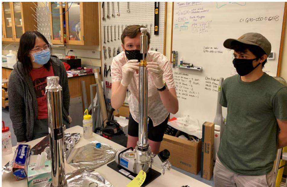
Figure 2. (From left to right) Students Judy Zhang, Matt Barickman, and Julian Rodriguez modifying a cryogenic trap to improve separation of noble gases for mass spectrometric analysis.
