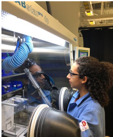
Figure 1. Fifth year PhD candidate, Sylvia L. Hanna, in the Farha group at Northwestern University handles air-sensitive, uranium-based MOF experiments in a glovebox under inert atmosphere.
