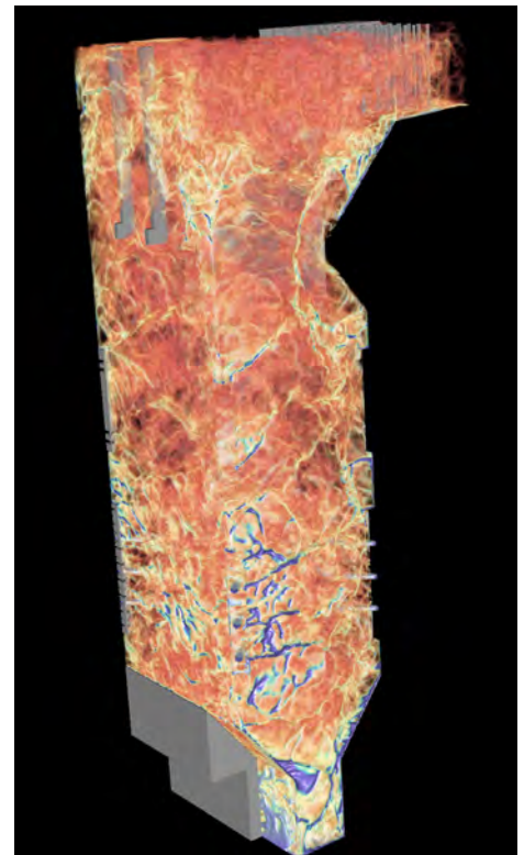
A volume rendered image of a CCMSC prediction of an Alstom oxycoal boiler. The image shows local concentrations of the 90 micron coal particles in the boiler. The particles concentrate in local regions due to variation in local Stokes number. The simulation was performed on Titan using 1 million core hours.
