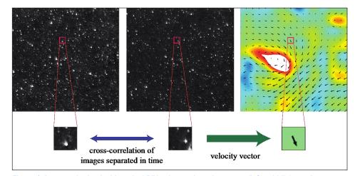
Figure 1. Images obtained with optical PIV, taken a short time apart (left, middle), can be subdivided into smaller images and cross-correlated to yield a velocity vector field from which quantities such as vorticity can be calculated (right).
