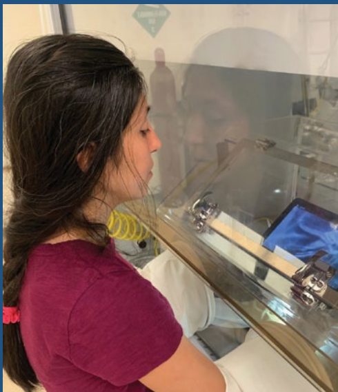
At the University of Illinois Chicago, Fatemeh Safari uses an inert atmosphere glove box to load an air sensitive sample into a diamond anvil cell for high pressure studies. A digital microscope provides for high magnification while allowing a wide field of view to aid in the loading process.
