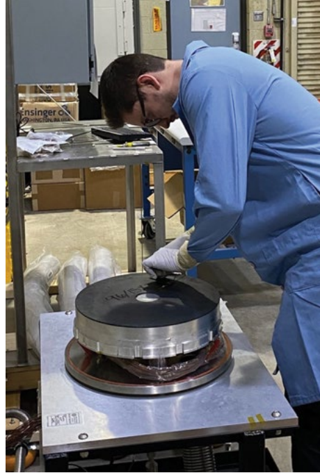
Figure 1. Placing thermocouples on a natural uranium plate to perform surrogate testing for the low-temperature experiments. The plate was cooled to -40^{\circ}\text{C} to test the thermal effects of the material.
