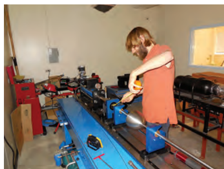
Figure 2. Avery Samuel prepares a high-strain-rate mechanical test using a split-Hopkinson pressure bar.
