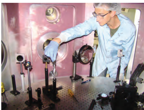
Figure 1. Graduate student Joe Strehlow sets up a Thomson scattering diagnostics at the Jupiter Laser Facility to validate a modeling prediction.
