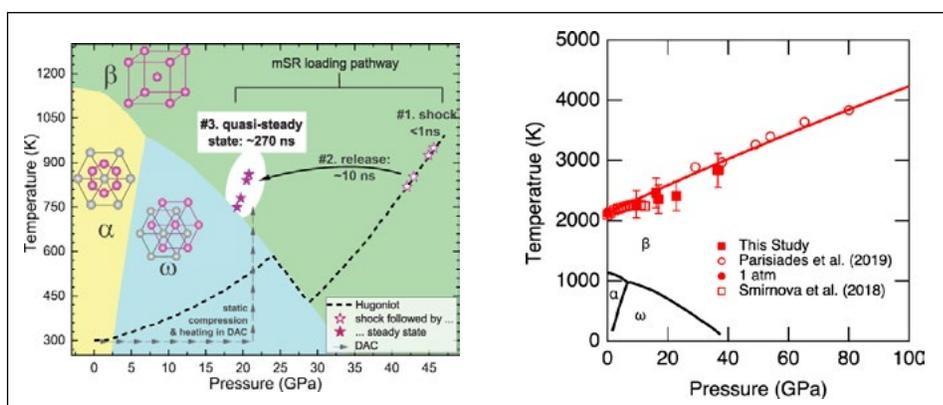
Figure 2. Left: P-T phase diagram and structural phase stability in zirconium studied using shock and DAC compression techniques and X-ray measurements at HPCAT and DCS.<sup>1</sup> Right: High pressure melt boundary of zirconium.<sup>3</sup>
