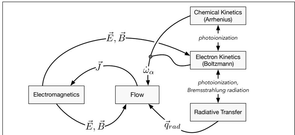
Figure 2. Overview of modeling schema mapping to underlying physics domains and primary coupling mechanisms.
