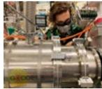
Chad Ummel couples the GODDESS ionization chamber to the scattering chamber containing the Oak Ridge Rutgers University Barrel Array (ORRUBA) in preparation for an experiment at the National Superconducting Cyclotron Laboratory.
