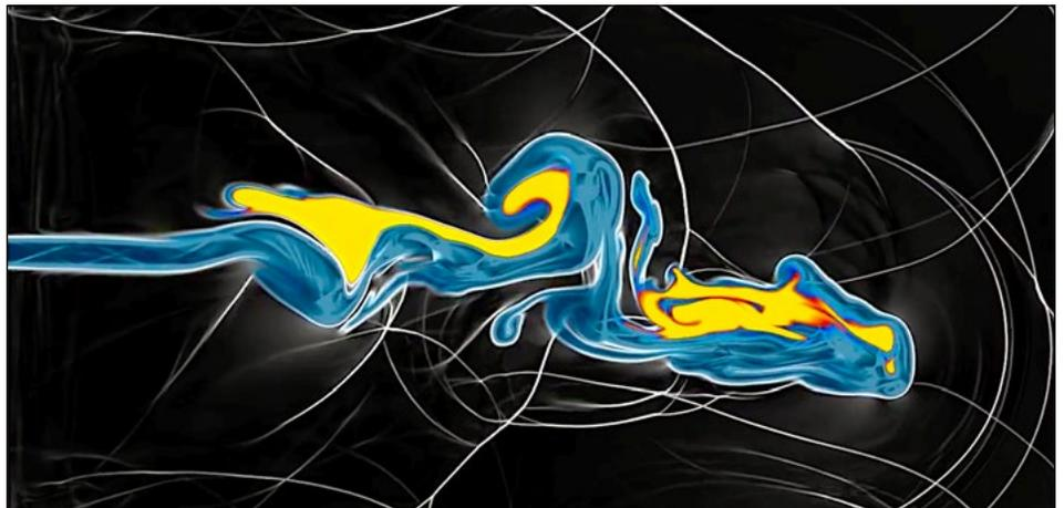
Figure 2. Preliminary simulations of laser-induced ignition using the Center's task-based simulation software (Courtesy of Dr. Mario Di Renzo and Dr. Kazuki Maeda).
