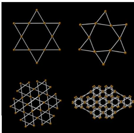
Figure 1. Kagomé net of Fe<sup>3+</sup> centers in jarosite. Top: Structural unit of the net at (left) ambient pressure and (right) 80 GPa. Bottom: Layers of extended nets at (left) ambient pressure and (right) 80 GPa.
