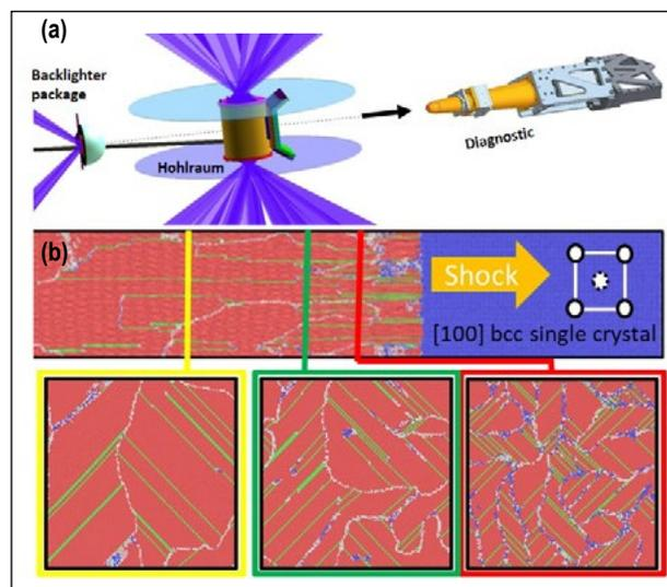
Figure 2. (a) Experimental setup at the NIF. Hohlraum is illuminated by 192 beams, and backlighter illuminates target for side-on radiography. (b) Molecular dynamics simulation of iron subjected to 55 GPa shock. The top image shows shock wave passing through single crystal bcc iron. The bottom image shows evolution of nanostructure as shock passes through. Colors represent different phases: blue = BCC, green = FCC, red = HCP, white = unidentified.
