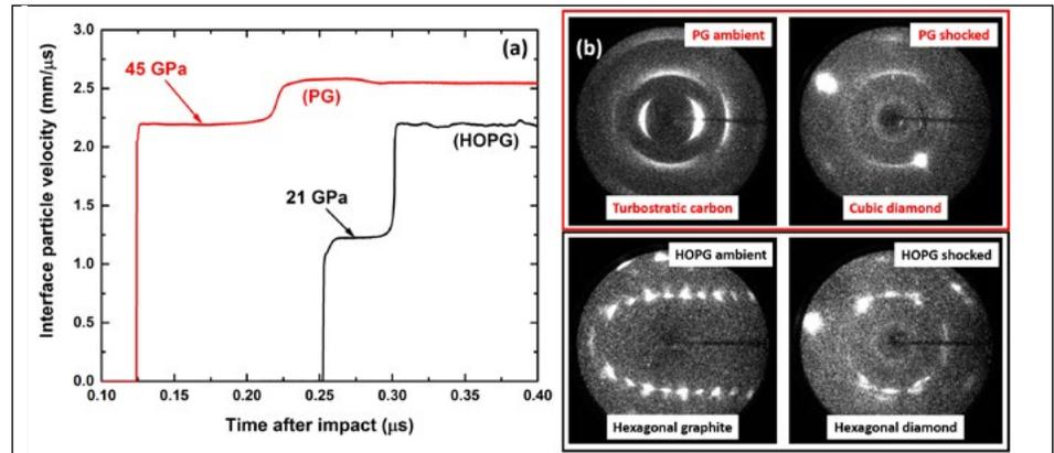
Figure 1. (a) Wave profiles and (b) XRD images from PG (red) and HOPG (black). Transformation stresses are labeled in (a), and the ambient and high-stress crystal structures are labeled in (b). Data in (a) and (b) are from Volz et al., J. Appl. Phys. 125, 245902 (2019), and Volz et al., Phys. Rev. B 101, 224109 (2020), respectively.
