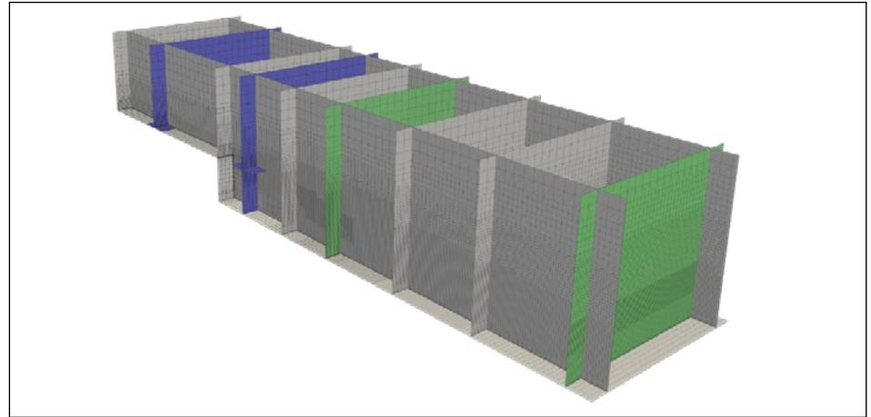
Figure 2. A computational grid for turbulence simulations produced by a grid-adaptation algorithm (i.e., without user input).
