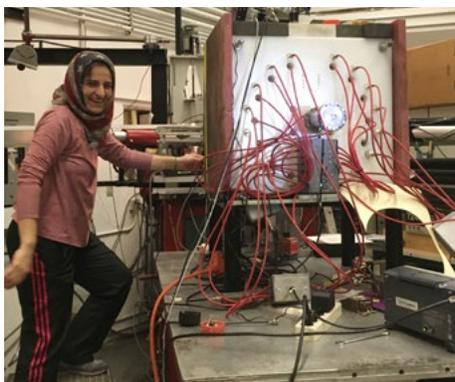
Figure 2. The HeBGB neutron detector for  $(\alpha, n)$  measurements.
