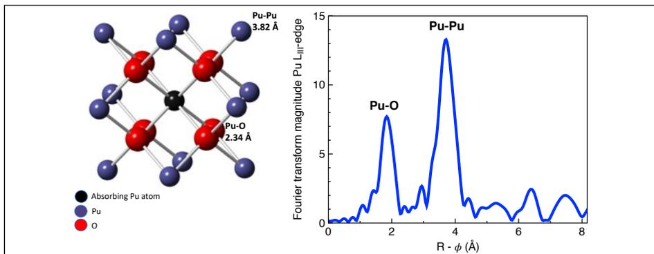
Figure 1. Extended X-ray absorption fine structure (EXAFS) spectra of a  $\text{PuO}_2$  sample that was corroded from Pu metal (left) showing peaks that correspond to the Pu-O and Pu-Pu shells of the  $\text{PuO}_2$  structure on the right.
