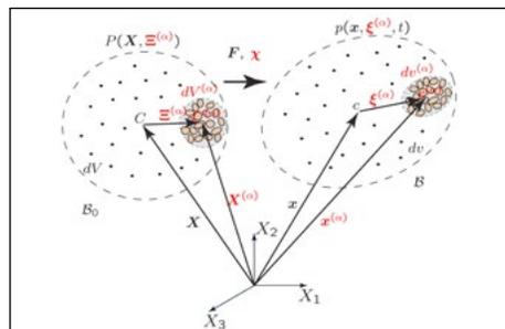
Figure 3. Illustration of mapping from reference to current configurations in micromorphic continuum field theories.
