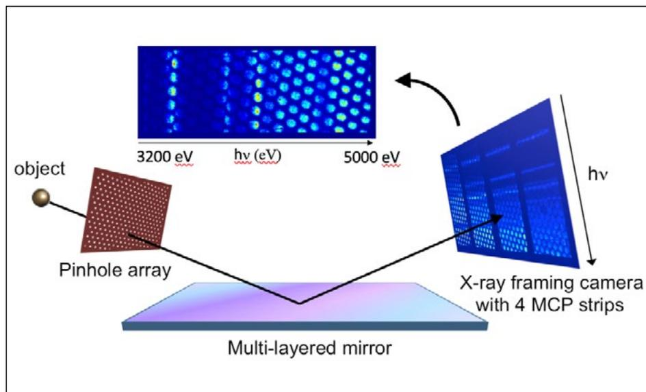
Figure 1. A multi-monochromatic imager, MMI, consists of a pinhole-array, multi-layered mirror, and microchannel plate (MCP), which records hundreds of object images with a horizontal photon-energy axis.
