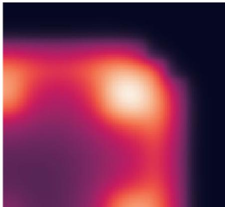
Figure 1. shows the power distribution in a quarter-core of a test reactor. I built this simulation from a time-dependent neutronics benchmark, and I use it to test and compare various numerical methods that can be useful in the transient simulation of reactors.
