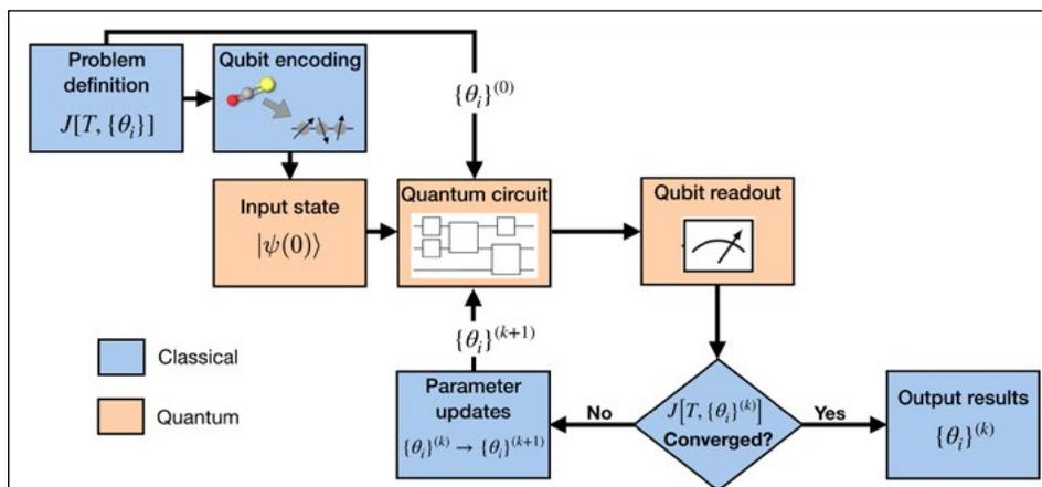
Figure 1. Block diagram of hybrid quantum-classical algorithm for designing parameterized laser fields to control molecular dynamics.
