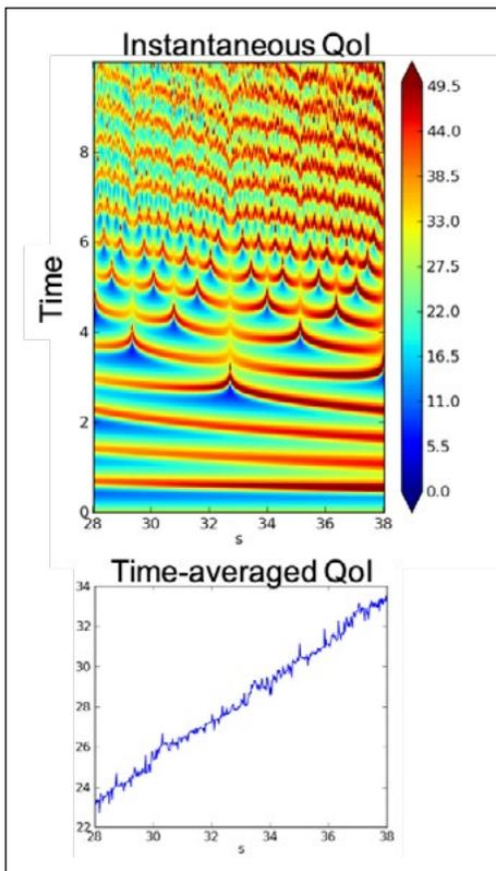
Figure 1. A sample Quantity-of-Interest (QoI) from the Lorenz system, illustrating the rapid decorrelation in time of nearby solutions (caused by differences in the parameters on the horizontal axis) which makes the problem of computing sensitivities of time-averaged QoIs an ill-posed problem (note the "noise" in the time-averaged QoI).
