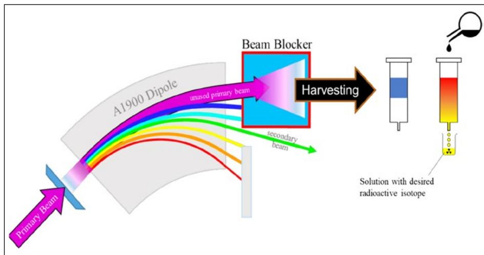
Figure 1. Graphic showing how isotopes will be produced and harvested from the FRIB facility at MSU with unused beam. Note that the secondary beam is the beam in which experimenters using the facility would be interested.
