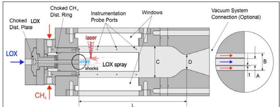
Figure 1. Computer-aided design schematics of the INSIEME experimental rocket-combustor geometry (courtesy of Carson Slabaugh, Purdue University).
