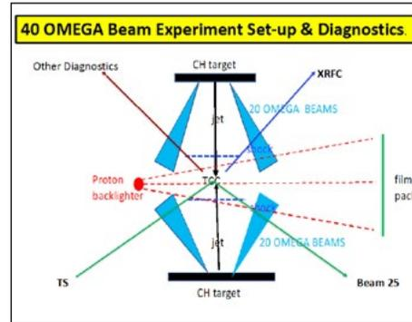
Figure 1. Sketch of experimental setup of colliding MG jets experiment using 40 OMEGA beams.
