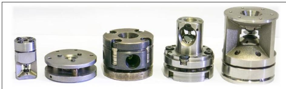
Figure 1. Various diamond anvil cell (DAC) platforms available and used for high-pressure experiments at HPCAT.
