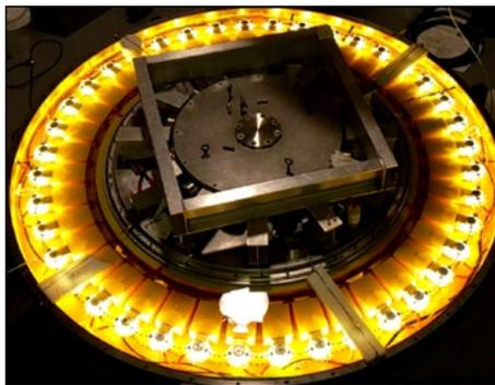
Figure 2. LTD Pulsed Power Machine MAIZE at the University of Michigan shown firing after being upgraded with 40 new switches.
