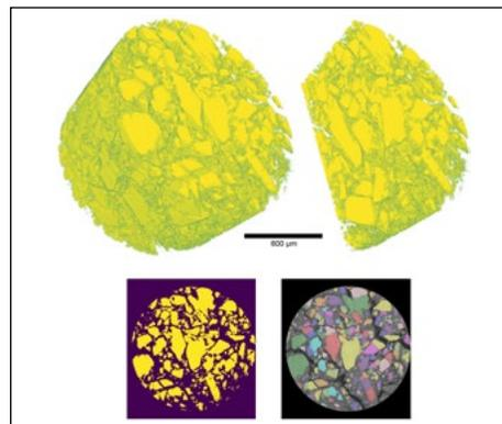
Figure 2. Computed Tomography (CT) image (top) of mock HE, courtesy of B.M. Patterson and J.D. Yeager (LANL), with watershed segmentation (bottom) by C.G. Becker and A.J. Clarke (Colorado School of Mines).
