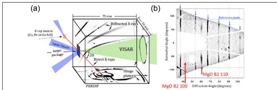
Figure 1. (a) Experiment geometry of the PXRDIIP diagnostic at the OMEGA-60 laser system. (b) *In situ* X-ray diffraction pattern of ramp-compressed MgO projected into  $\phi$ - $\chi$ - $\delta$ -spacing coordinates. Observed peaks demonstrate formation of the high pressure B2 phase of MgO.
