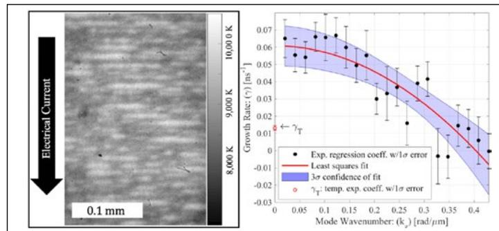
Figure 1. Left: ETI perturbations are seen in the aluminum-6061 surface temperature (from a 3- $\mu$ m/3.5-ns-FWHM-resolution image). Right: ETI exponential growth rate vs perturbation wavenumber.
