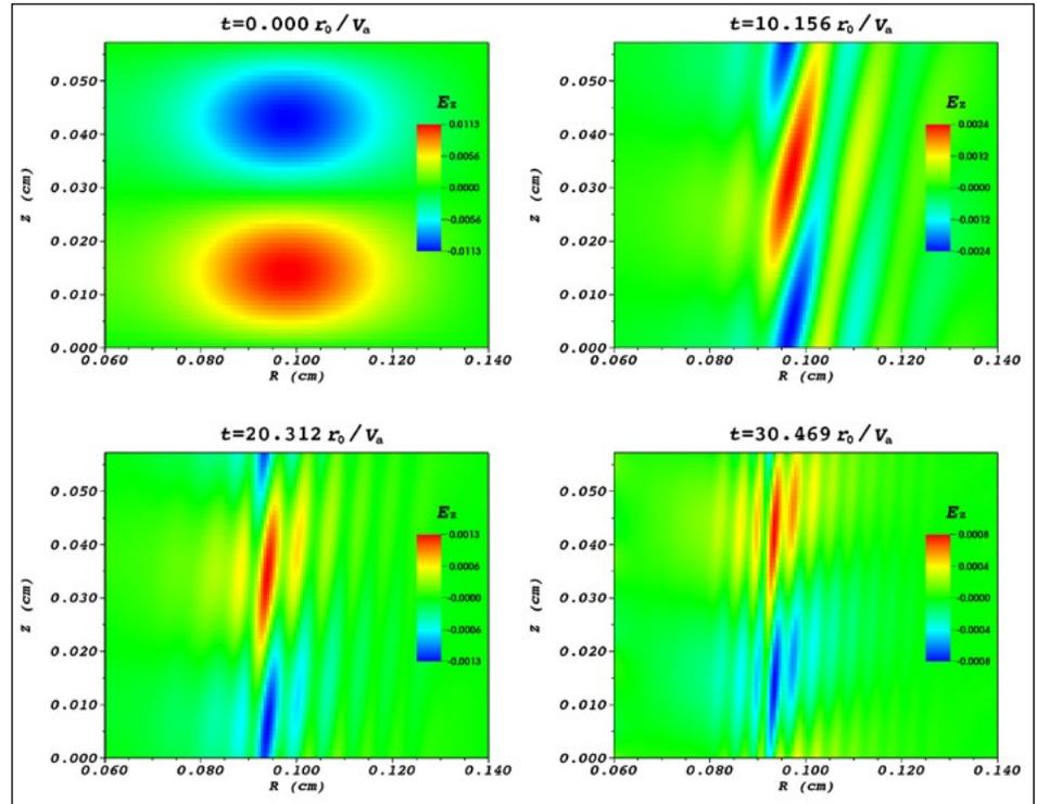
Figure 1. Snapshots of the time evolution of the seeded perturbation in a SFS Z-pinch. Each plot illustrates spatial distribution of the normalized axial electric field of the perturbation in the RxZ plane. Flow shear stretches and smears the perturbation, so that no exponential growth is observed, and the pinch is stabilized against a linear mode of a given axial mode number  $r_0 k_z = 10$ , where  $r_0$  is the pinch characteristic radius.
