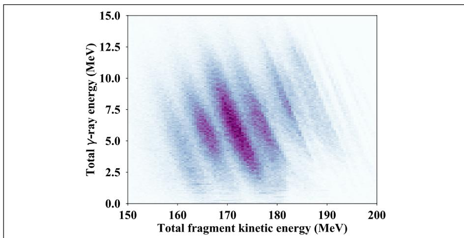
Figure 1. Calculated correlations between fission fragment kinetic energies and total  $\gamma$ -ray energy emitted by the fission fragments.
