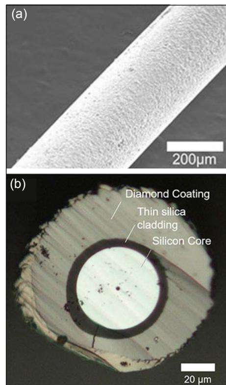
Figure 2. (a) Scanning electron microscope image of diamond encapsulated silicon fiber showing homogeneous morphology. (b) Cross section of a 50 micron silicon fiber after polishing in an ion mill. The fiber is clad in a thin layer of silica and coated in diamond.
