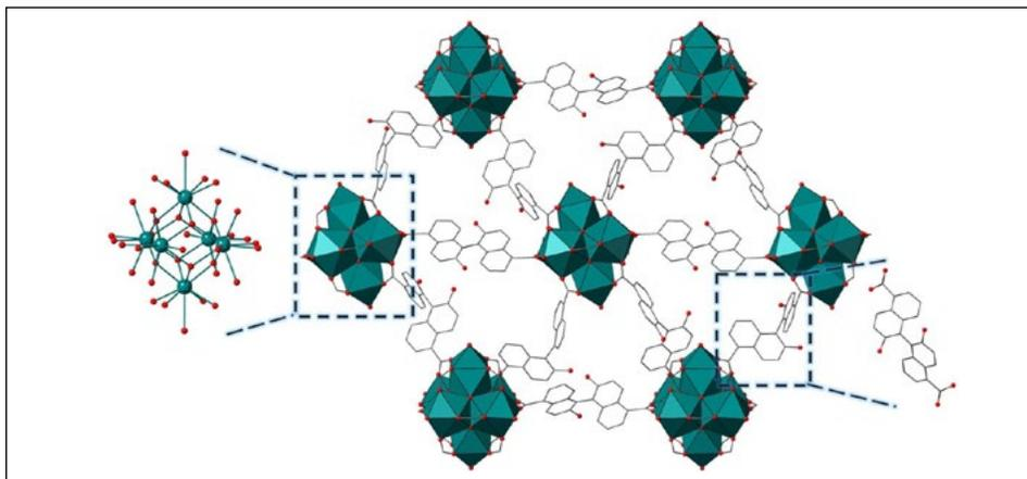
Figure 2. The structure of the new thorium-based MOF that holds the record of being the most radiation resistant.<sup>3</sup> The structure consists of thorium oxide nodes (shown on left) and binaphthol linkers (right). Th, O and C are shown in blue, red, and grey, respectively.
