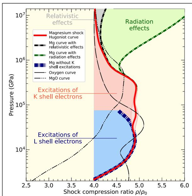
Figure 1. Shock Hugoniot simulation for magnesium is compared with results for oxygen and magnesium oxide. Densities are divided by the initial density of  $\rho_0 = 1.737 \text{ g cm}^{-3}$ . The broad temperature interval from 250,000 to  $1.6 \times 10^7$  K, where the Mg curve exceeds a compression ratio 4, can be attributed to ionization of the K and L shell electrons. Relativistic and radiation effects only become important at the highest pressures.
