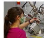
University of Notre Dame postdoctoral scholar Danielle Hutchison preparing to collect single-crystal X-ray diffraction data for an actinide compound at high pressure in a diamond anvil cell.
