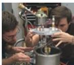
Graduate students Maxwell Sorensen and Austin Abbott (CENTAUR, TAMU) inserting a parallel-plate avalanche counter into a testing chamber.
