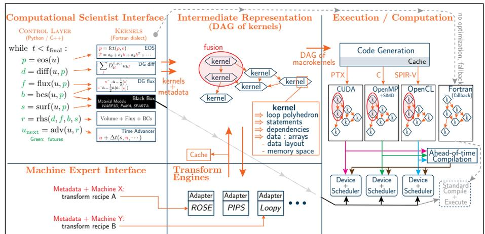
Figure 2. The MIRGE computer science framework, designed to balance usability (with python-based control layer) against portability, which is facilitated by the abstractions of the intermediate representation and existing hardware-targeted code-generation tools.
