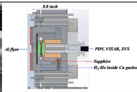
Figure 1. (Left) Assembled pre-compression cell in a stripline geometry for a Z experiment. (Right) Schematic of a pre-compression cell (2 inches wide and 0.8 inch tall). The fluid mixture of hydrogen-helium is captured inside the copper gasket placed in between two sapphire anvils.
