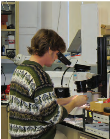
Eugene Vinitzky, a student from the California Institute of Technology and a participant in Carnegie's Summer Scholars Program, prepares a diamond anvil cell for measurements of the Raman spectra of BaReH9 at high pressure. Vinitzky's stay at Carnegie was supported by the Carnegie-DOE Alliance Center. He is now a graduate student in Physics at the University of California-Santa Barbara.
