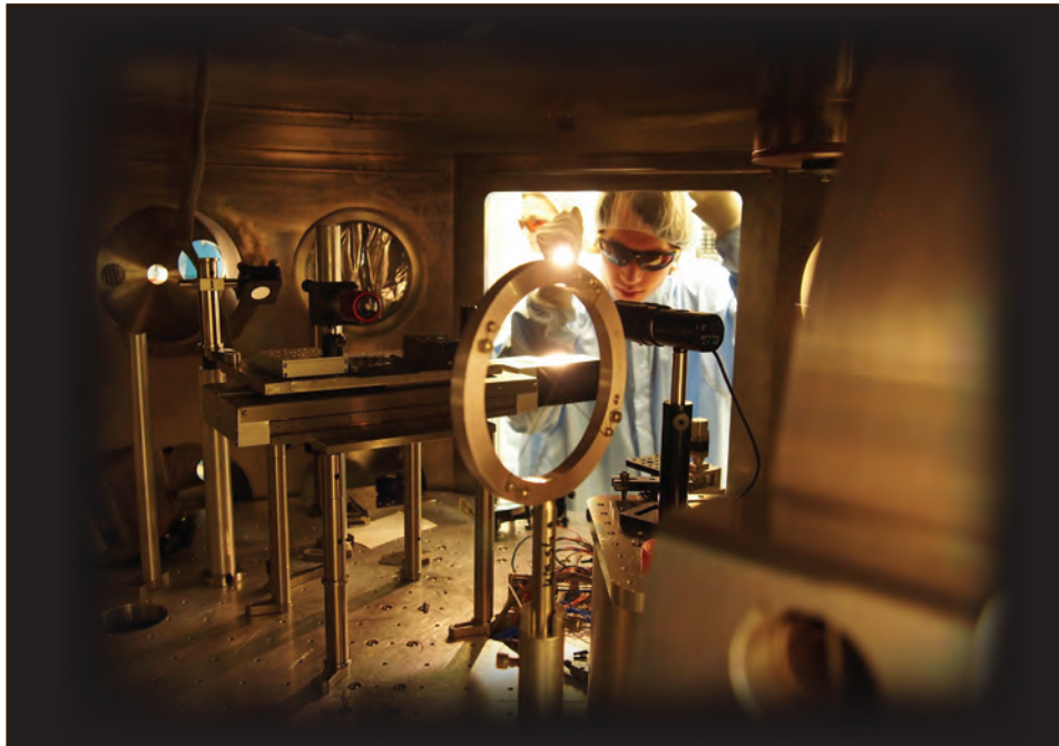
The Texas Petawatt Laser high intensity target chamber from behind the final mirror.
