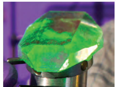
Figure 2. The unique High Explosives Crystal Laboratory at LANL creates and provides samples for critical property measurements for these materials. Shown is a crystal about the size of a golf ball illuminated by laser light—representative of some of the laser techniques used to measure elasticity for this study. (Photo credit: Ethan Froggett)
