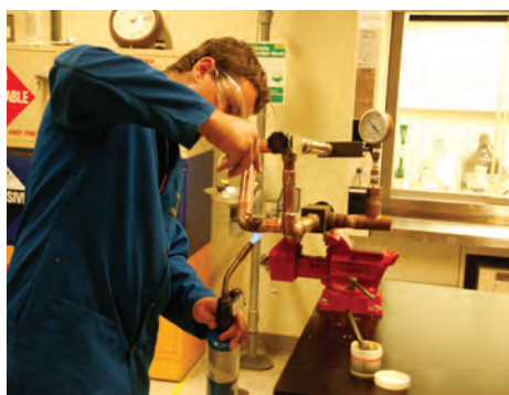
Physics undergraduate student, Zackary Rehfuss, assembling a pumping system for a dilution refrigerator in the laboratory of Professor Brian Maple at UC San Diego. The dilution refrigerator will be used to cool high pressure cells down to millikelvin temperatures for electrical transport and magnetic measurements on f-electron materials at high pressures into the megabar range.
