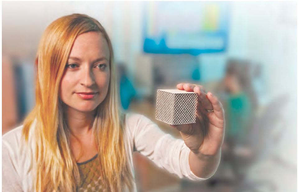
Figure 1. Materials scientist Holly Carlton holds an additively manufactured metal lattice structure. A combination of modeling and synchrotron radiation microtomography experiments helped identify and correct some initial printing problems compromising structural integrity. 1 (Photo by George Kitrinis.)
