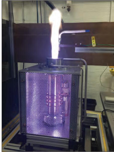
Figure 1. The 50 kW inductively-coupled plasma torch in the Flowfield Imaging Lab at The University of Texas here shown operating with air as the feed gas.
