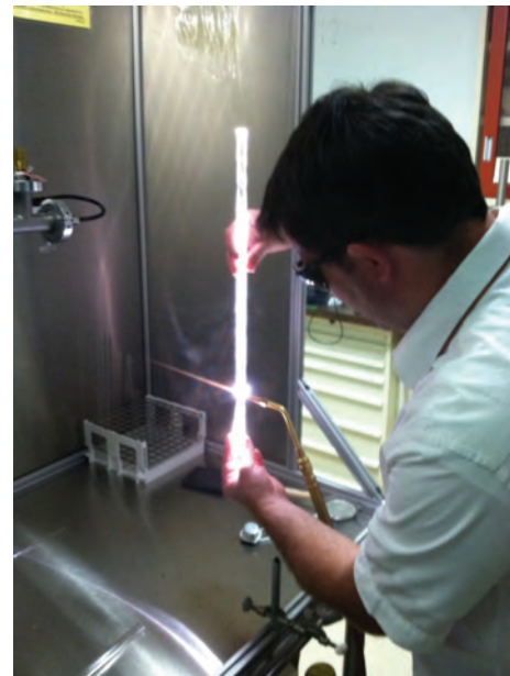
Figure 2. Quartz-tube sealing is a capability key to a variety of sample synthesis efforts supporting LLNL missions ranging from basic science to forensics to global security.
