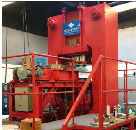
Figure 1. The 2000-ton, multi-anvil, high pressure apparatus installed in the High Pressure Lab at Stony Brook University.
