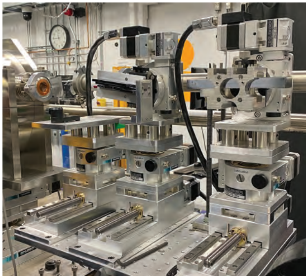
Figure 1. Single Multilayer Monochromator System in the Laser Shock Station.
