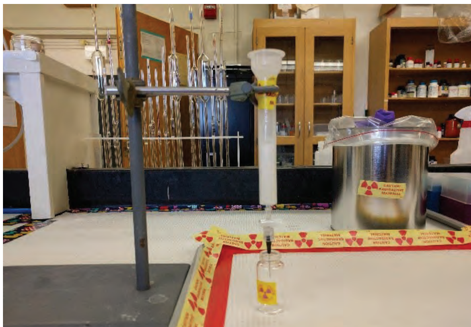
Figure 1. ^{99}\text{Mo} is loaded onto the column and ^{99\text{m}}\text{Tc} may be eluted from the column as the ^{99}\text{Mo} decays.
