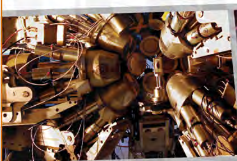
▲ Germanium Array for Neutron-Induced Excitations at Los Alamos Neutron Science Center - courtesy of Los Alamos National Laboratory
