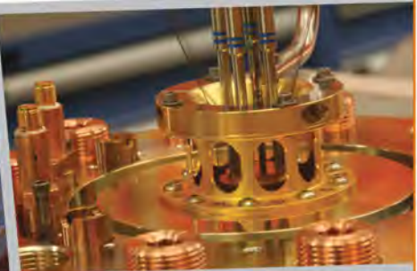
▲ A z-pinch wire array is prepared for shooting on the Z inertial confinement fusion facility at Sandia National Laboratories in New Mexico - courtesy of Sandia National Laboratories
