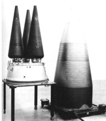
Figure 46. W-78 Warhead. Deployed on Minuteman III missiles, they are reaching end of life and are to be replaced by W-87-1 warheads.
