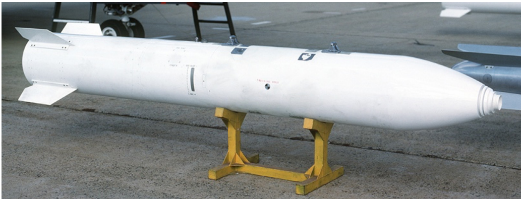
Figure 48. B-83 Modern Strategic Bomb. They are deployed aboard strategic bombers. Physically, they are the largest weapon in the stockpile and have the largest yield.
