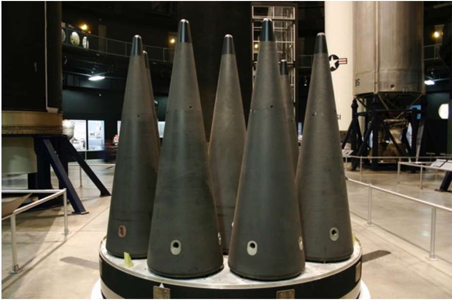
Figure 50. W-87 Warhead. It was deployed originally on the MX Missile (shown here), and is now deployed on the Minuteman III missile.
