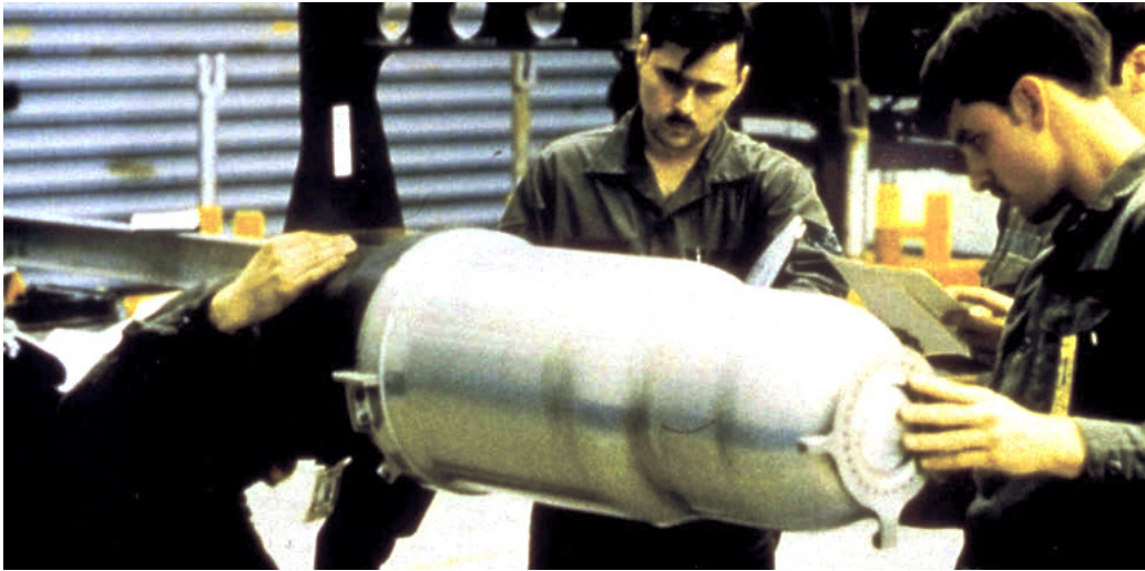
Figure 47. W-80 Warhead. They are deployed on Air Launched Cruise Missiles aboard strategic bombers. In 2021, they are undergoing life extension to be deployed on the future Long Range Stand-Off missile.
