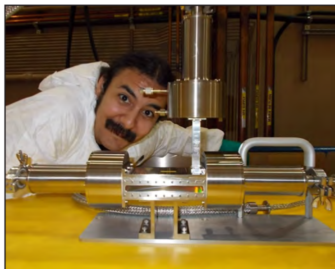
Figure 2. Gas cavity for measuring the optical properties of white dwarf stars. Ross Falcon graduated in 2014 from UT-Austin with a PhD in Astronomy and is now a postdoctoral researcher at Sandia.
