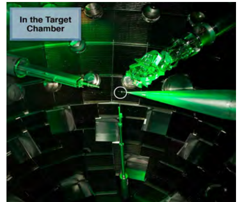
Figure 1. Target assembly for a shock-timing target held in place by the cryogenic cooling target positioner system (left image). View inside the NIF chamber of a target inserted on the positioner system as well as several diagnostic arms (right image).
