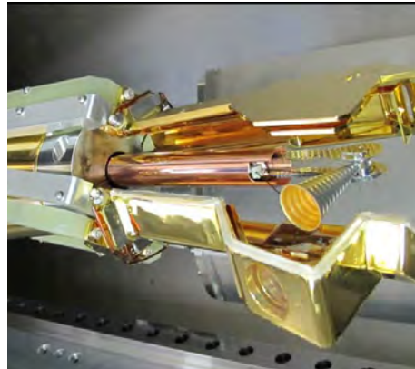
Figure 1. Target assembly for a shock-timing target held in place by the cryogenic cooling target positioner system (left image). View inside the NIF chamber of a target inserted on the positioner system as well as several diagnostic arms (right image).
