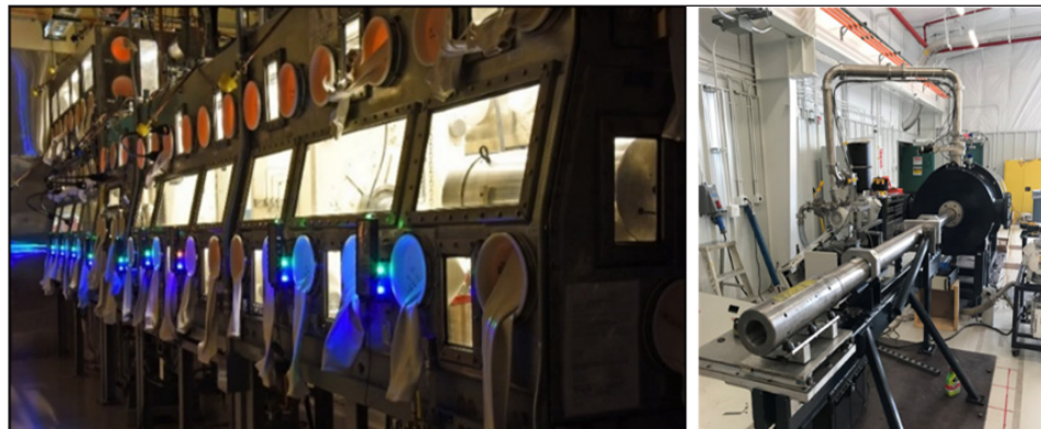
Figure 1. Photo of the TA-55 40 mm gun and glove box (Left) and the 40 mm powder gun at DEOS (right). The DEOS 40 mm gun is the test bed for developing new experiments and diagnostics prior to being conducted on the TA-55 40 mm gun.
